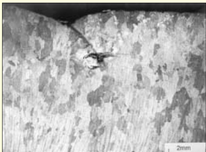
Figure 4: Macroetched Sample with Inclusion Defect Near Oscillation Mark.
