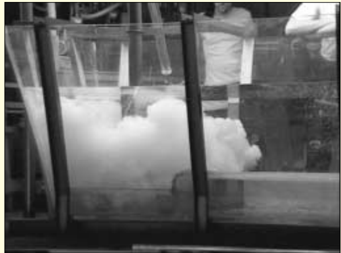
Figure 8: Particle Injection into Tundish Water Model through Shroud.
