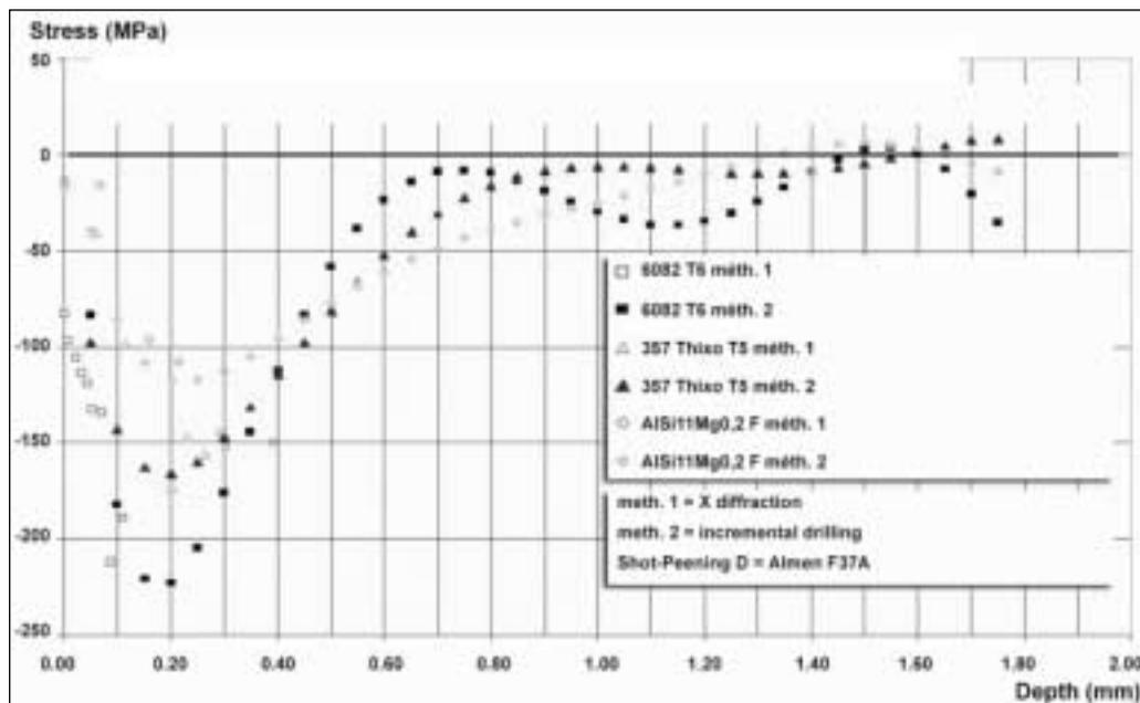
Fig. 10 – Residual stress measurements after shot peening.
