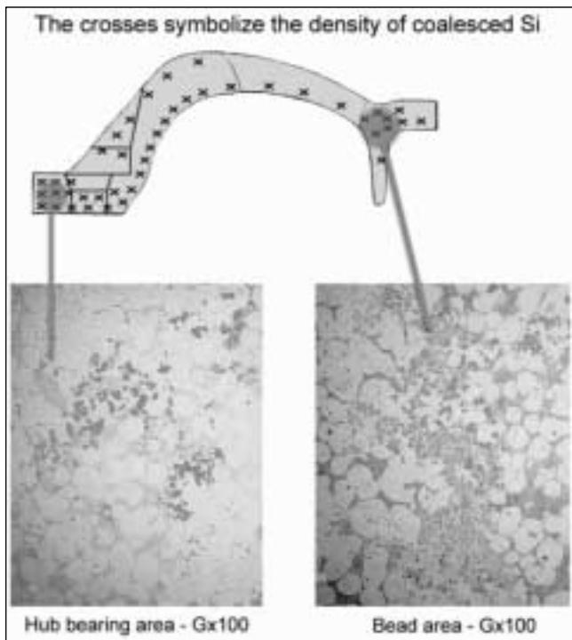
Fig. 7 – Thixoformed AlSi7Mg 0.6 T5 alloy disc. Coalesced silicon.
