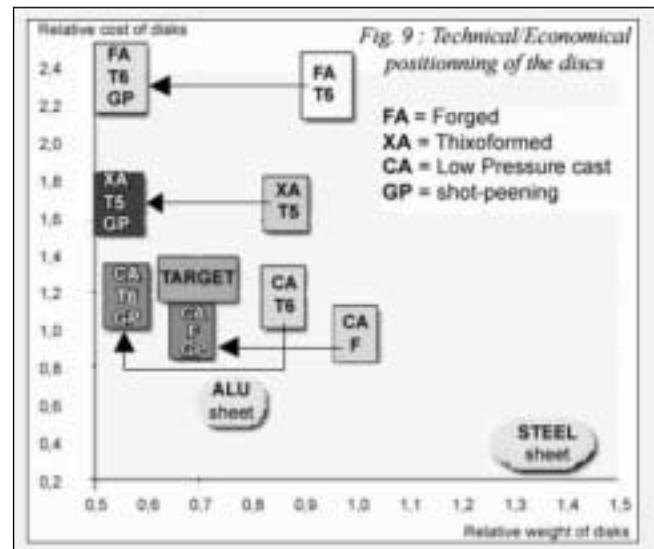
Fig. 9 - Technical/economical positioning of the disc.
