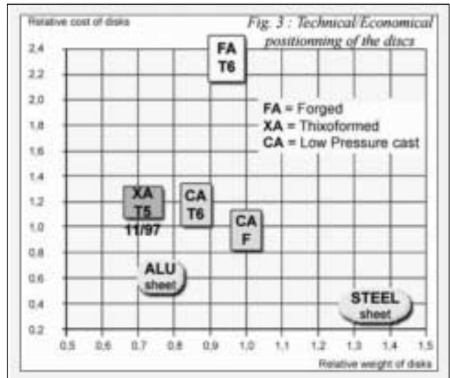
Fig. 3 – Technical/economical positioning of the disc.
