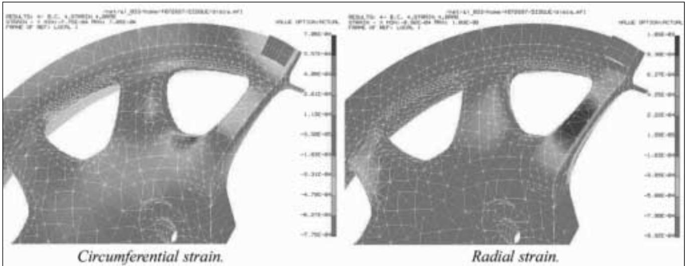
Fig. 2 – Computer models of disc strain.
