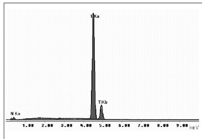
Fig. 2 – Plot of the X-ray dispersive energy spectrometer measurement from the droplet surface developed on the TiN/(Ti,Al,Si)N/TiN.
