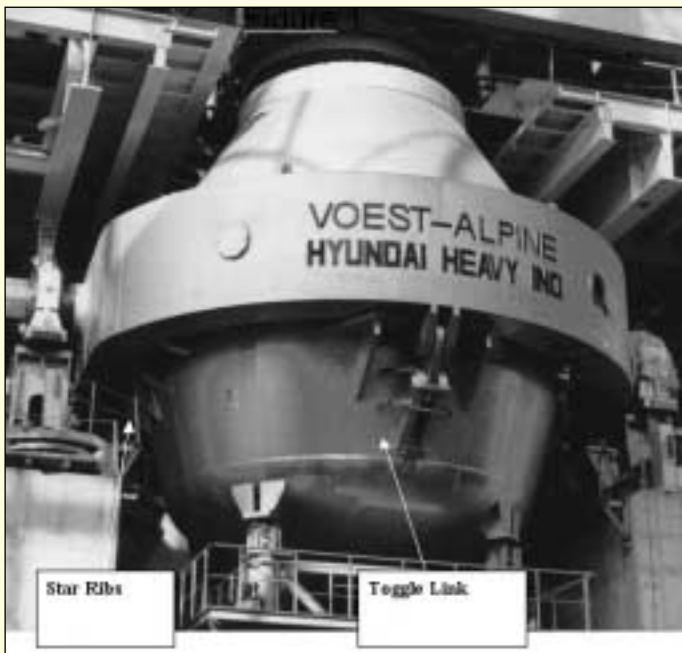
Figure 1: 300-ton LD Converter with VAI-CON ® Disk Suspension System Showing the Toggle-Link, POSCO Kwangyang Works, Korea
