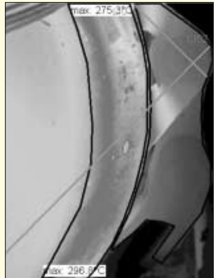
Figure 7: Temperature Profile of a Horizontal Link Assembly (ISPAT ISCOR Vanderbijlpark, South Africa).
