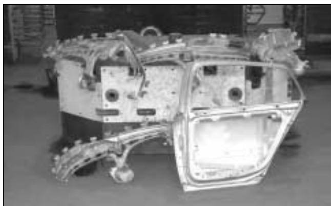
Fig. 3 - Struttura portiera pressocolata. Fig. 3 - Inner door panel for car makes in die casting.
