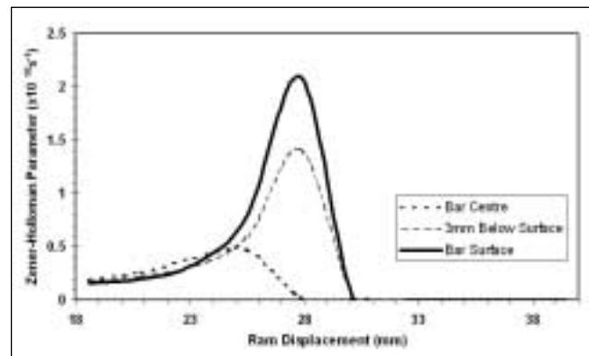
Figure 4: The Zener-Holloman parameter for three of the points tracked through the die
