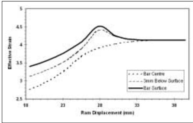
Figure 5: Effective strain for three of the points tracked through the die
