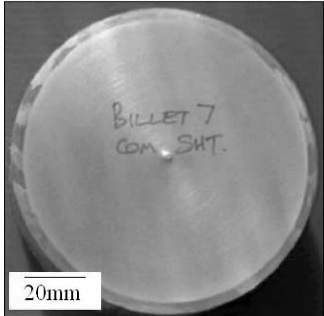
Figure 1: Macro-etched slice from flat die extruded bar
