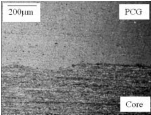
Figure 2: Optical micrograph showing the PCG boundary
