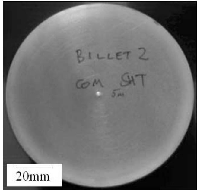
Figure 7: Macro-etched slice from Die X extruded bar
