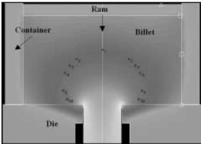
Figure 3: A snapshot showing the configuration of the finite element model with the start point of the point tracking.
