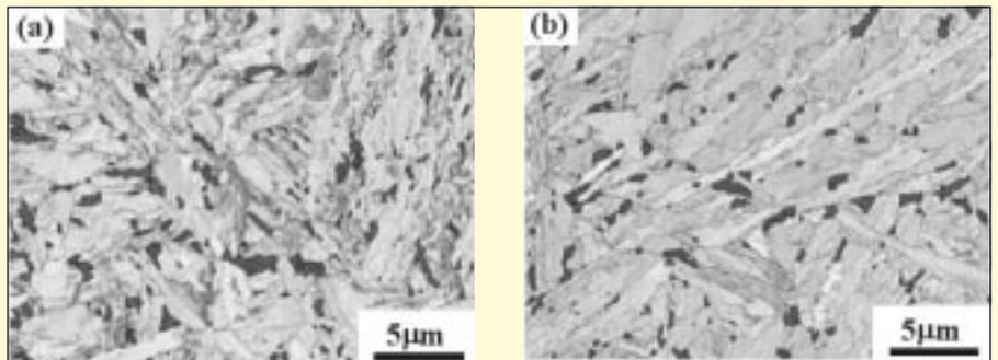
Fig. 9 – OIM maps of specimens tempered at 650 °C for 1 h (a) without field and (b) with a 14-T magnetic field. The field direction is horizontal in the picture [34].
