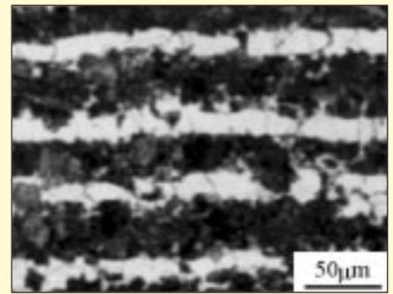
Fig. 5 - Banded microstructure in 42CrMo obtained by conventional annealing (the rolling direction is horizontal in the picture) [29].
