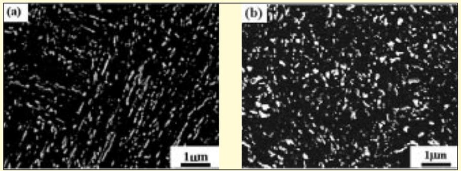
Fig. 7 – SEM micrographs of carbide obtained by being tempered at 650 °C for 1 h (a) without magnetic field; (b) with a 14-T magnetic field. The field direction is vertical. SEM secondary electron images [34].
