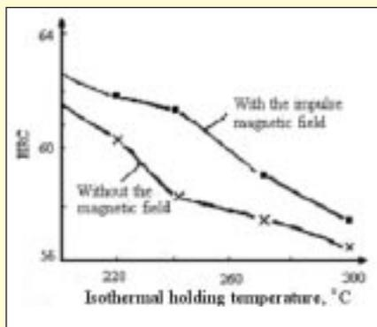
Fig. 3 – Hardness of 9SiCr as a function of isothermal holding temperature [21].
