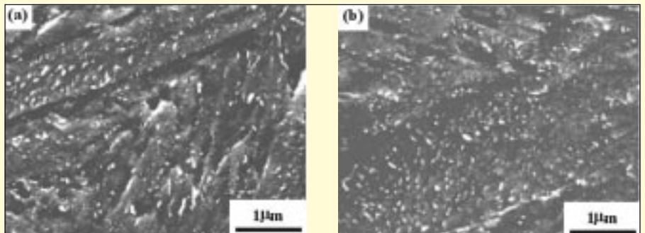
Fig. 10 – SEM secondary electron images of carbide precipitates (bright areas) within martensite in specimens tempered at 200 °C for 60 min (a) without and (b) with a 14-T magnetic field (the magnetic field direction is vertical in the micrograph) [35].
