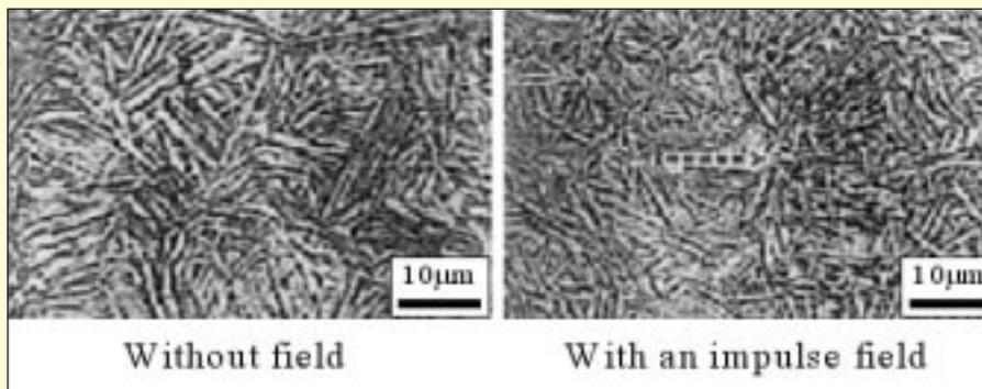
Fig. 2 – Bainitic microstructures of 9SiCr isothermal quenched at 300 °C for 45min without and with the impulse magnetic field [21].
