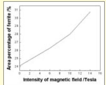
Fig. 6 - Influence of magnetic field on the amount of ferrite [32].
