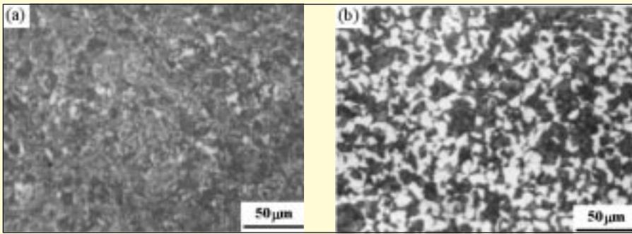
Fig. - 4 Microstructure of specimen heat treated at 880 °C for 33min and cooled at 46 °C/min without (a) and with (b) a 14-T magnetic field, Field direction is vertical in the picture [32].
