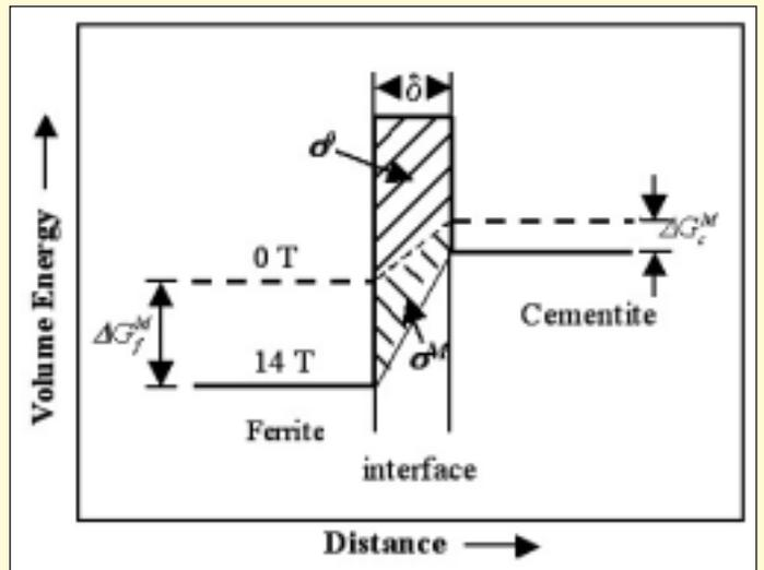
Fig. 8 – Schematic illustration of cementite/ferrite interfacial energy without and with the magnetic field.
