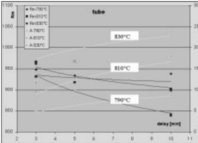
Fig. 6 – Ultimate tensile stress ( $R_m$ ) (blue curves, left y-axis) and toughness (yellow curves, right y-axis) versus delay at bainite transformation temperature.
