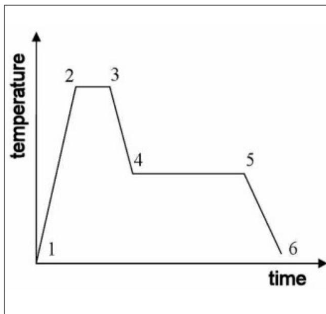
*Fig. 1 – Diagram of heat treatment of TRIP steel:
