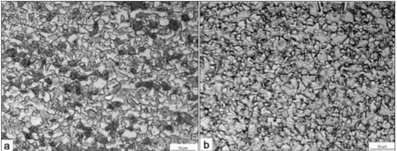
Fig. 2 – Microstructures upon intercritical annealing: (a) after quenching to water, (b) after delay at 410°C; etched with Nital and 10% aqueous solution of  $\text{Na}_2\text{S}_2\text{O}_5$  (bright gray ferrite, dark martensite and bainite, white austenite).
