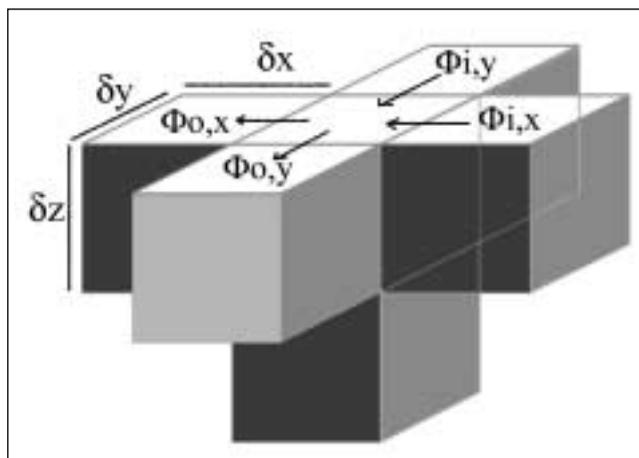
Fig. 1 – Scheme of the cells and heat flows for rectangular ingots.
