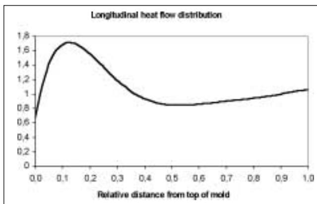
Fig. 2 – Normalized heat flow distribution along casting direction.
