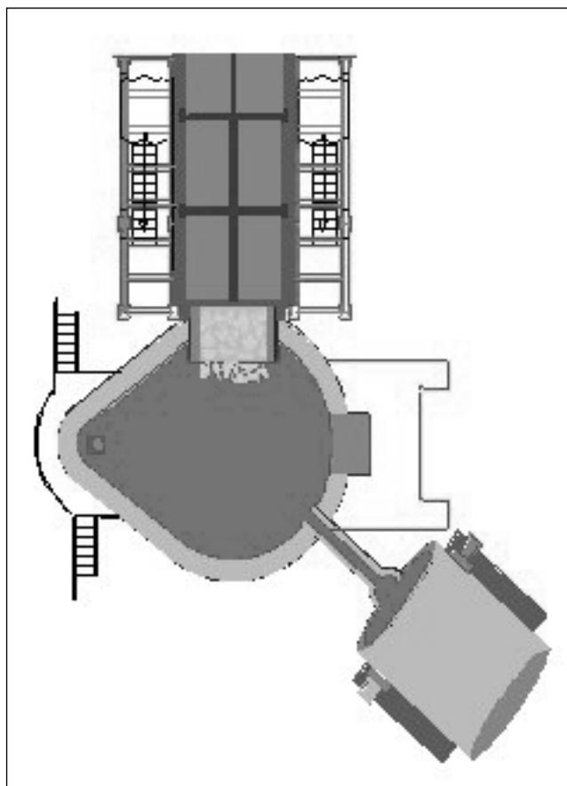
Fig. 9 – Hot metal charging concept – plan view.
