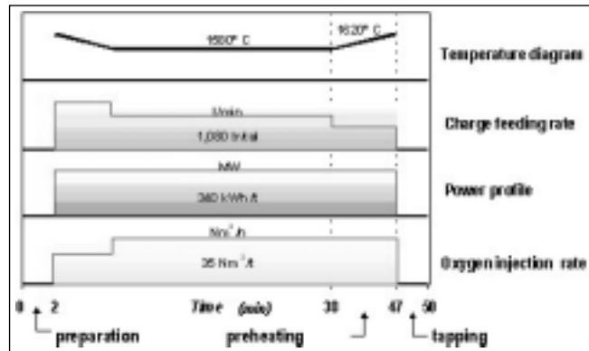
Fig. 6 – Consteel® heat cycle.
