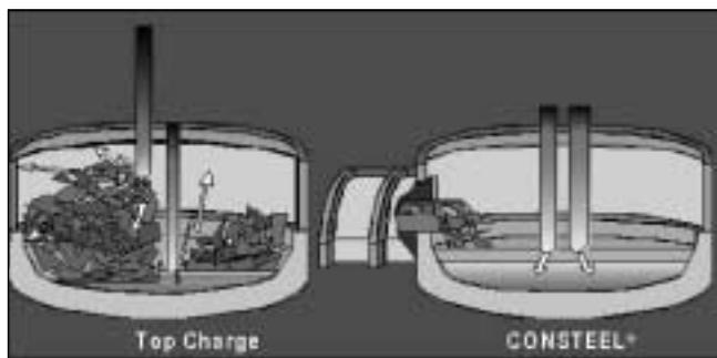
Fig. 7 – Scrap charge on a batch-type top-charged furnace and on Consteel® system.
