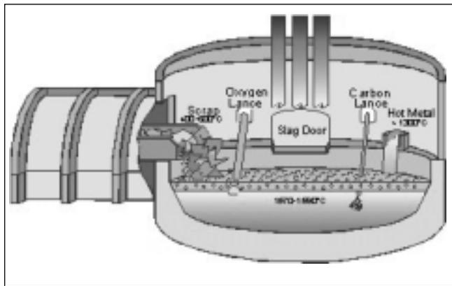
Fig. 10 - Hot metal charging concept - side view.
