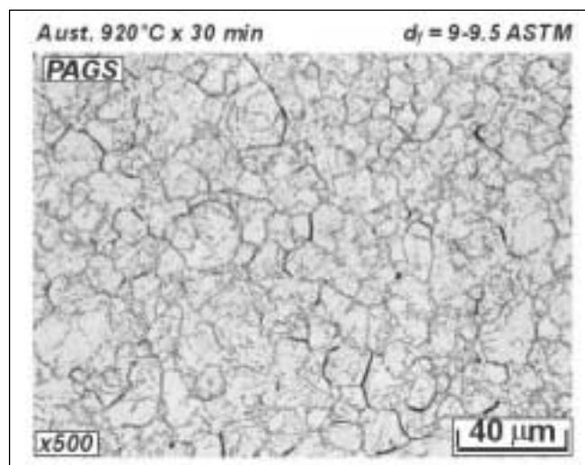
Fig. 10 – Mo-Ni-Nb-V Steel. AGS obtained with austenitizing temperature of 920°C and quenching with CR = 12°C/s. Prior austenite grain boundaries were revealed by selective etching by saturated picric solution.
