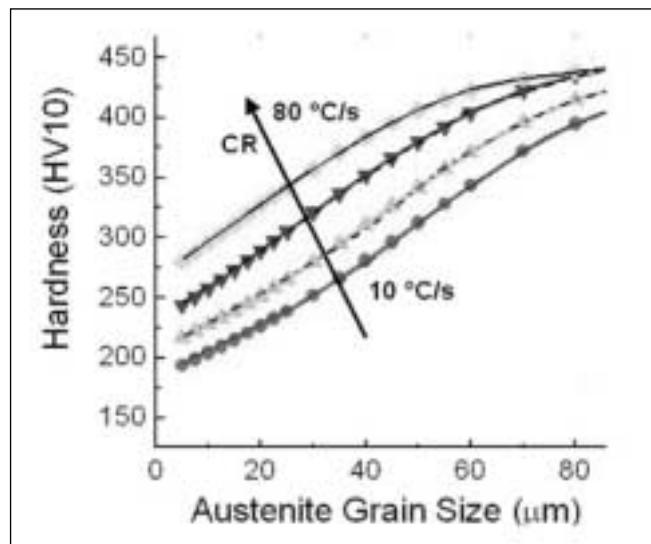
Fig. 3 – Calculated effect of AGS and cooling rate during quenching on hardness.
