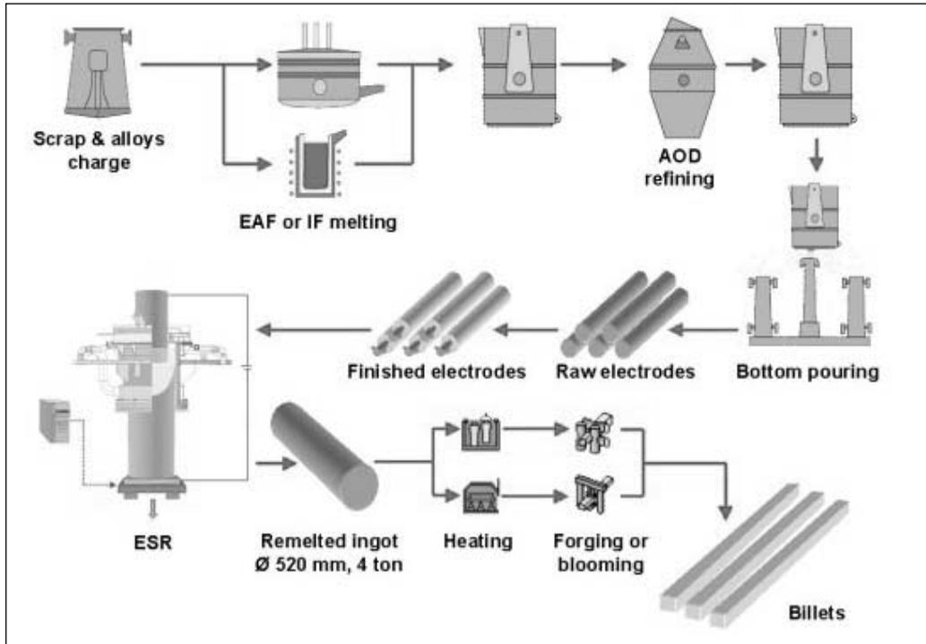
Fig 2 – The complete ESR production cycle.
