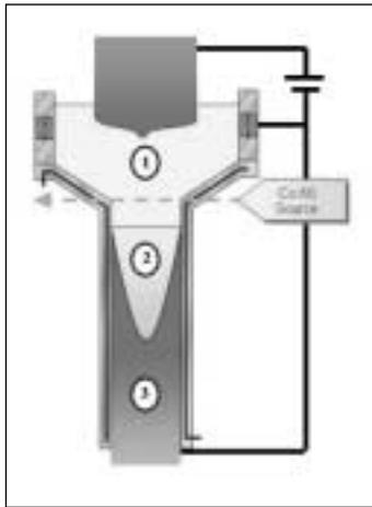
Fig. 4 – The ESRR® mould during process.
