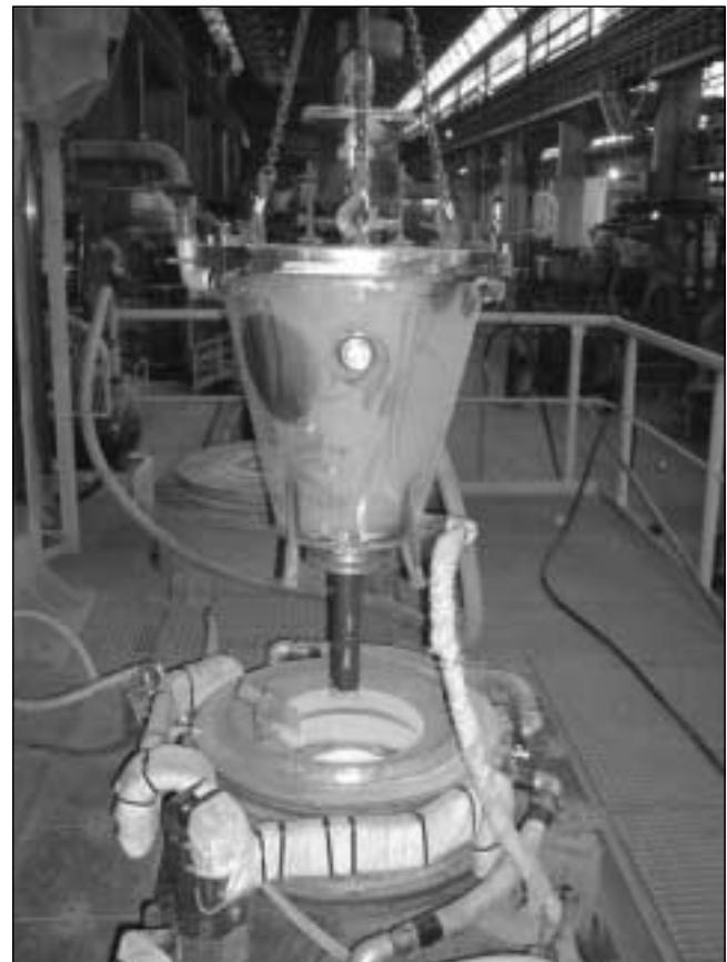
Fig. 10 – The slag suction device ready to operate.
