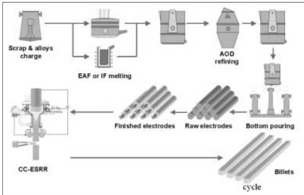
As soon as the billet reaches its required length, a powder cutting torch (oxygen + iron powder injection) automatically cuts the billet which is then removed in an unloading position. The revolutionary innovation is that all the continuous production of up to 40 billets in one remelting sequence out of multiple of electrodes.
