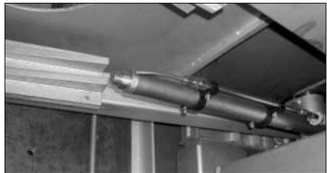
Fig. 17 – Overview of the cutting device, with the swivelling torch, the water spray system for the granulation of the generated slag and protection of the copper box.
