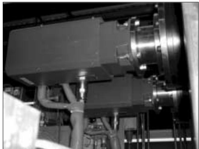
Fig. 16 – The brushless electrical engines that drive the rolls.
