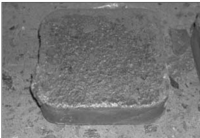
Fig. 19 – A sample slice cut by the oxygen-powder torch. Note the good surface.
