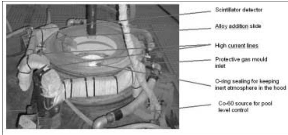
Fig. 5 – The complete mould assembly during CC-ESRR® process.
