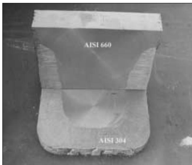
Fig. 20 – Transversal and longitudinal section of the transition zone.
