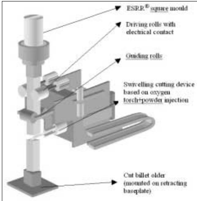
Fig. 13 – The CC-ESRR® manipulator schematics.
