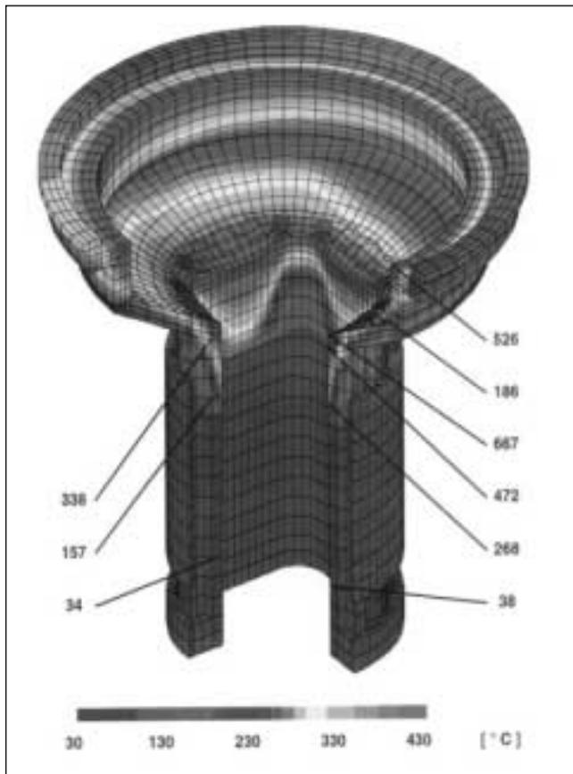
Fig. 9 – FEM analysis of the mould during the process: the mould temp. distribution. Photo Courtesy of INTECO / AVL LIST.
