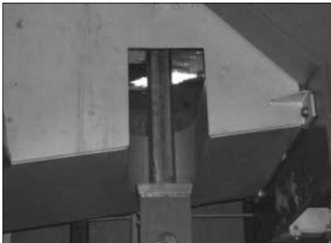
Fig. 18 – The cutting device during operation. Note the billet and the billet holder are mounted on the retracting baseplate.
