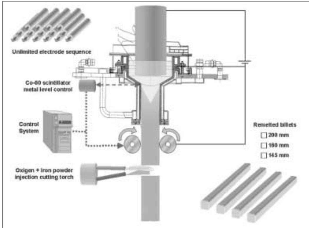
Fig. 12 – The complete CC-ESRR® production cycle.
