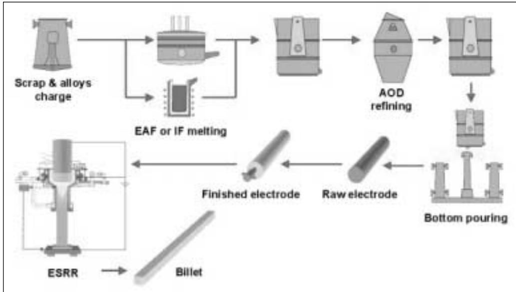
Fig. 8 – The complete ESRR® production cycle.
