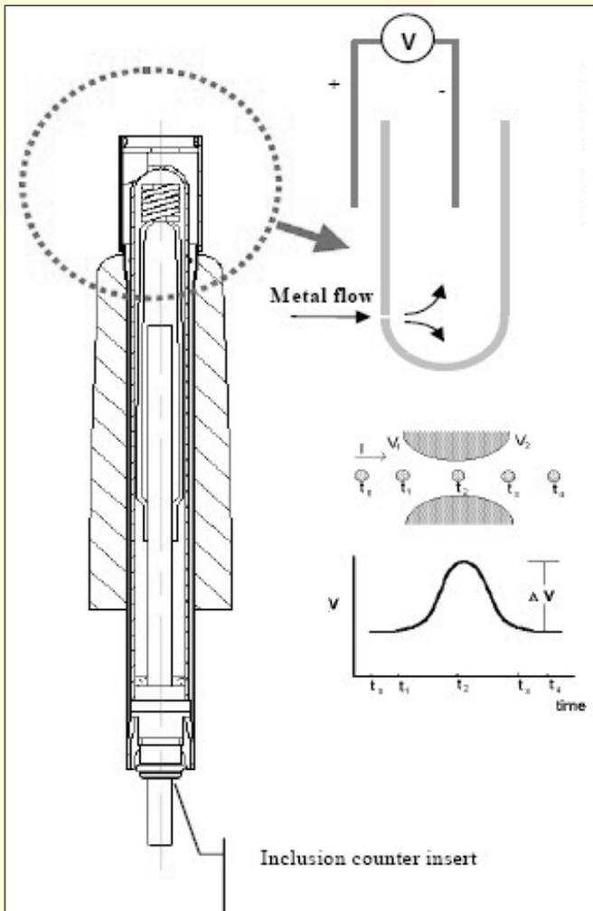
Fig. 9: Functional principle of the Inclusion Counter.
