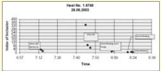
Fig.10: Inclusion Counter measurements in ladle metallurgy.
