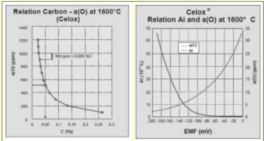
Fig. 1e: Relations oxygen activity vs. %carbon and %Al vs. EMF.
