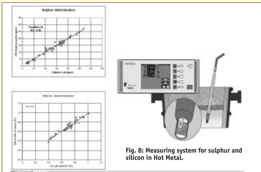
Fig. 8: Measuring system for sulphur and silicon in Hot Metal.
