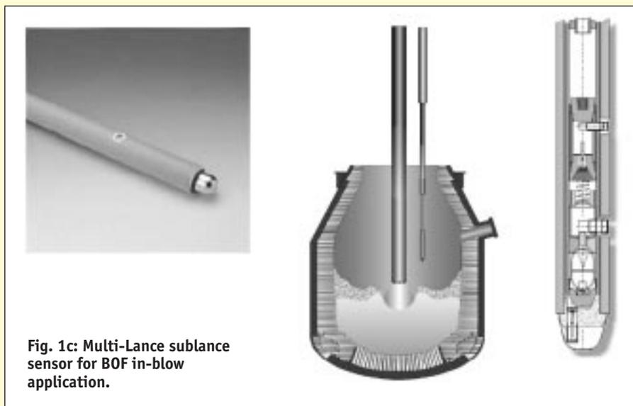
Fig. 1c: Multi-Lance sublance sensor for BOF in-blow application.
