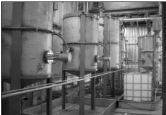
Fig. 11 – Impianto pilota processo pirometallurgico c/o AST. Fig. 11 – Pilot plant of pyrometallurgical process c/o AST, Terni.
