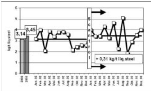
Fig. 13 – Gunning consumption before and after implement SCANTROL™\*.
