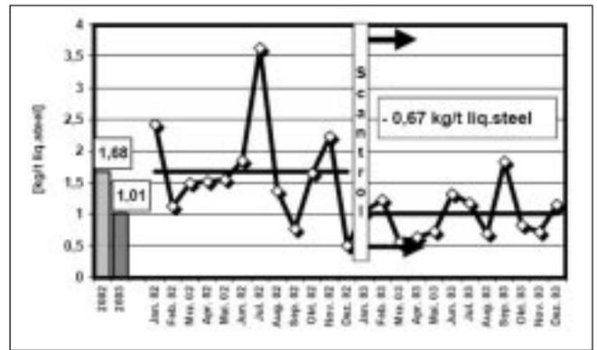
Fig. 14 – Bottom/bank cold repair consumption before and after implement SCANTROL™\*.
