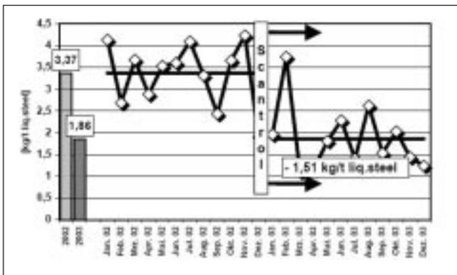
Fig. 12 – Brick consumption before and after implement SCANTROL™\*.
