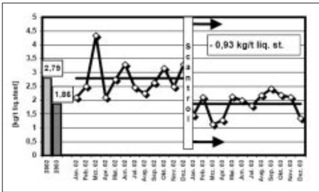
Fig. 11 – Refractory maintenance time before and after implement SCANTROL™\*.
