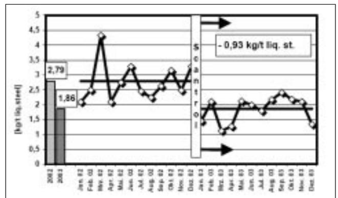
Fig. 15 – Bottom/bank hot repair consumption before and after implementation of SCANTROL™\*.
