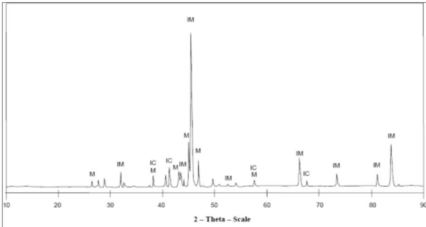
Fig. 7 – XRD of ferromanganese alloy produced from the smelting of manganese ore sinter fines cold bonded with 9% cement addition.
