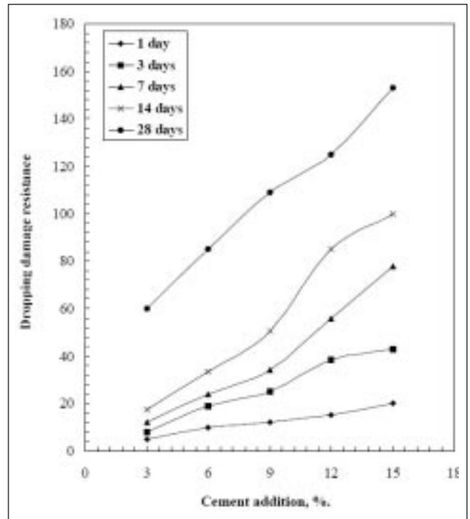
Fig. 3 – Effect of cement addition on the dropping damage resistance of pellets cured at different curing periods, (water amount = 10%).
